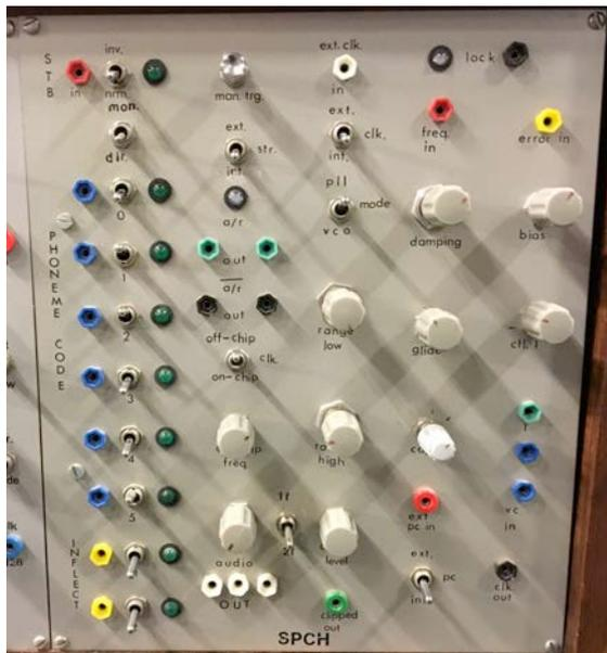
**Figure 11: The Phoneme Generator module, with XOR'ed switches and input bits at left**
