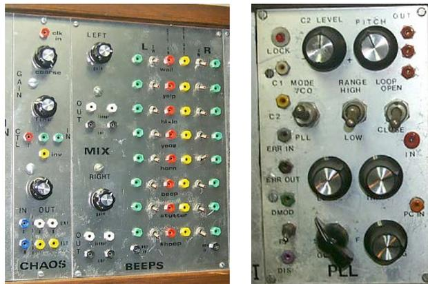
**Figure 10: The Voltage-Controlled Chaos and Alarms Modules (left) and a Phase-Locked Loop (Right)**
