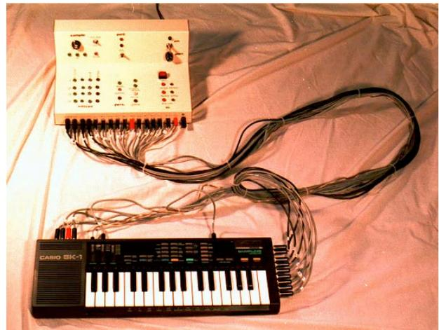
Figure 12: The SKI and its standalone Interface module
