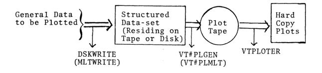
B) <u>Plotting with VT#PLGEN and DSKWRITE</u>: In order to preformat your data for plotting with VT#PLGEN, the DSKWRITE/ HEADER/FINISH subroutine package must be used. (To access these routines, use: \$ASSIGN1 LIB=VT%LIBRY DIR=VT%DIRCT before an \$EXECUTE GO or CATALOG).
